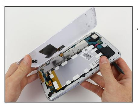
Once the backing has been pried off all around the device, remove the white backing.
