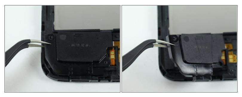
After detaching the connector and removing the screw, carefully remove the right speaker using tweezers.
