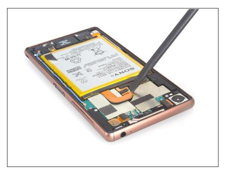
Release battery flex connector carefully to avoid breaking the pins.
