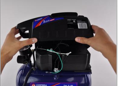
Remove the plastic shroud from the compressor.
