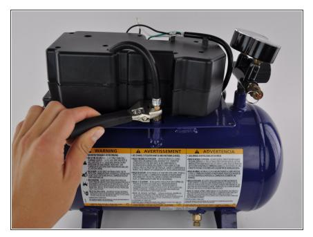
Unscrew the exhaust tube from the check valve using a Smart Wrench.
