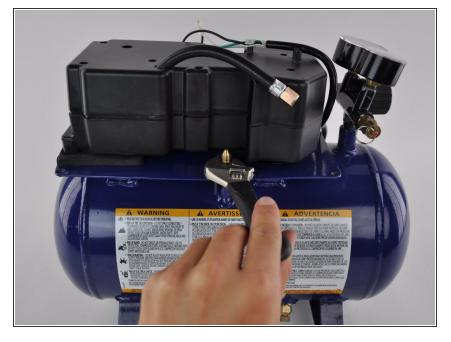
Unscrew the check valve by twisting it counter-clockwise using a Smart Wrench.
