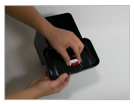
Grip either in the inside or outside of the switch with the needle nose pliers or your hand, and pull to remove the switch.
