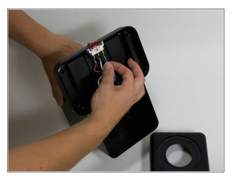
Use your hands or a pair of needle nose pliers to remove the wire attached to the switch.
