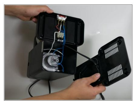
Remove the bottom cover from the machine and slide it down the power cord.
