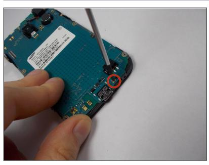
Use a philips-head screwdriver to remove the single screw on the bottom of the phone.
