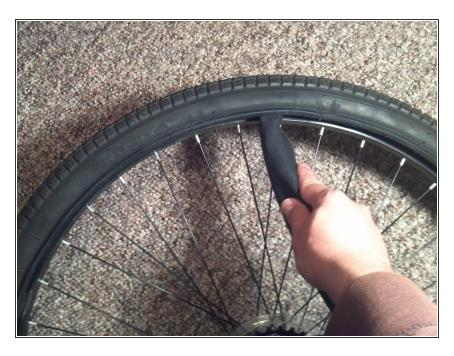
Starting at the valve, pull the inner tube out of the gap between the rim and the tire.
