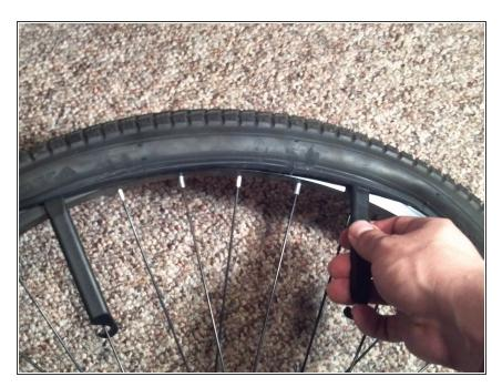
• Insert one tire lever under the tire and hook it onto a spoke. Insert the other tire lever next to the first and slide it along the rim to remove one side of the tire from the rim.
