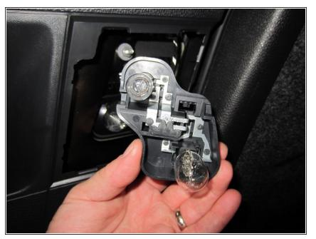
• Turn the assembly so that the smaller tail light bulb and larger fog light bulb are visible.
