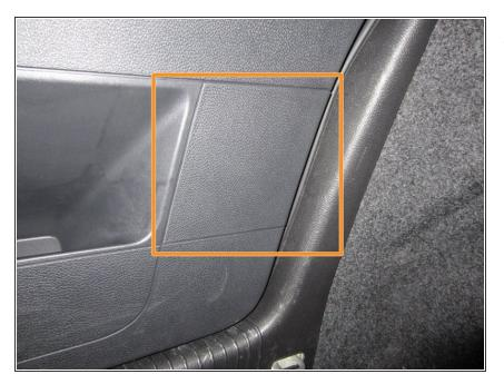
On the driver's side of the vehicle's rear cargo area, locate the rectangular tail light compartment cover.
