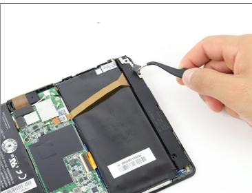
Peel off the stickers holding the left speaker in place with a tweezer or by using your fingers
