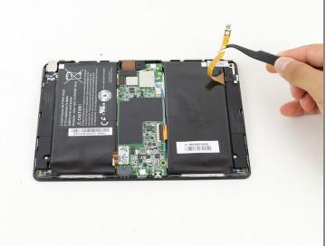
• Remove the battery connector using either your fingers or a pair of <u>tweezers</u>.
