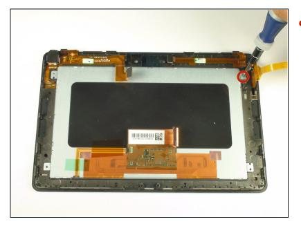
Remove the one remaining Phillips screw holding the display in place.
