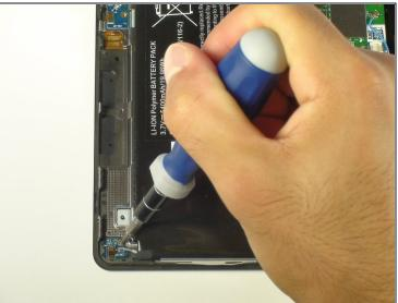
• Unscrew the small blue boards in each corner with the same Phillips screwdriver.
