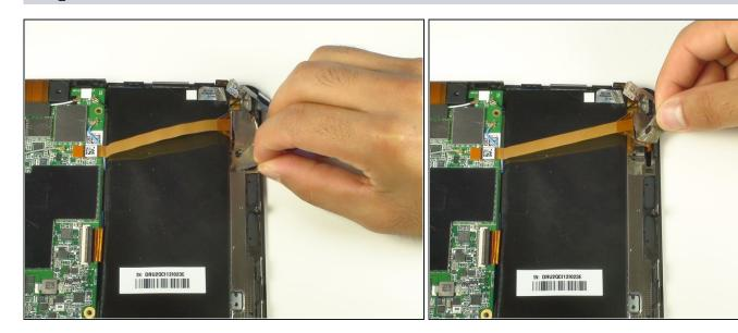
Remove the sticker holding the touchscreen controller in place to free it from the midframe.
