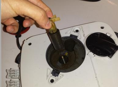
Firmly lift the impeller up and out of its casing.
