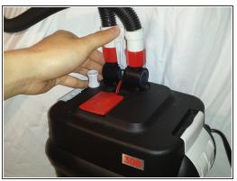
• Lift AquaStop Valve lever all the way up. This will stop the water flow and preserve the vacuum so that there shouldn't be a need to prime the filter again.
