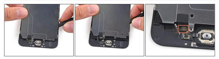
• Slide the point of a spudger behind the shield plate to gently lift the home button cable up off of the front panel.
