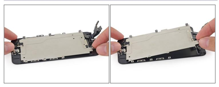
Lift the front-facing camera end of the LCD shield plate up slightly.
