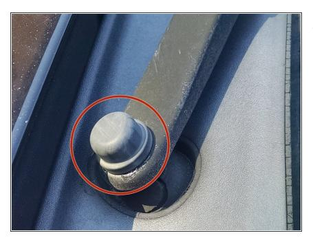
Use a plastic prying tool or spudger to gently remove nut cap from wiper base.
