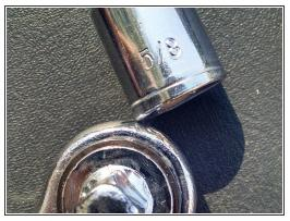
• Use a 5/8 wrench or socket to remove the necessary nut holding the wiper in place.
