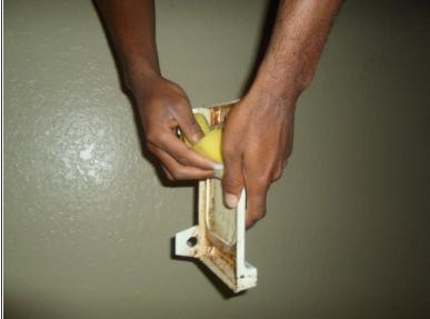
• The evaporator tray might have ice build up on it. You can remove this ice by pouring warm water on the tray. After the ice is melted, clean the tray with warm water and soap.
