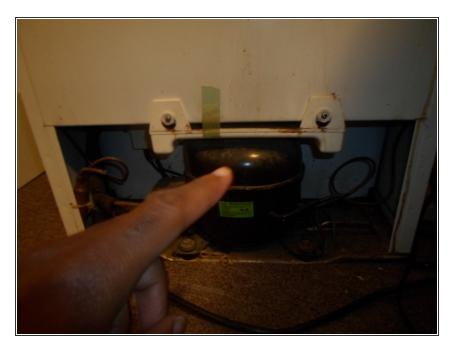
Go to the bottom of the back side of the refrigerator and locate the cut out where the compressor and evaporator are stored.
