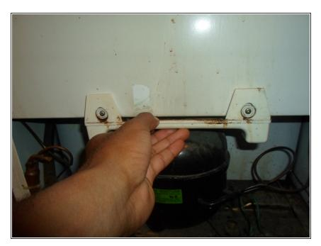
Remove the evaporator tray by simply pulling up and out the tray. make sure that none of the liquid spills.
