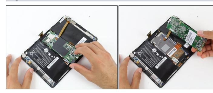
• Gently lift the motherboard away from the device. If there is any resistance, check the previous steps to ensure that all connections have been removed.
