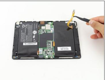
• Remove the battery connector using either your fingers or a pair of <u>tweezers</u>.
