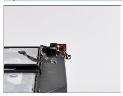
Remove the 5 mm Phillips screw securing the IR board to the optical drive bracket.
