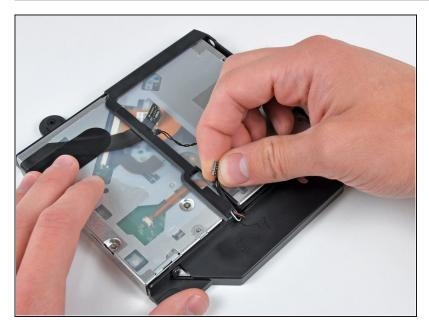
Carefully de-route the IR sensor cables from the channel in the optical drive bracket.
