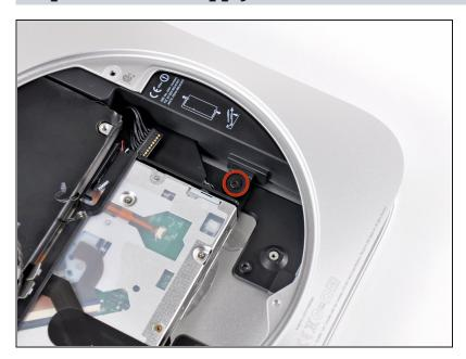
Remove the 7.9 mm T6 Torx screw securing the power supply and optical drive to the outer case.
