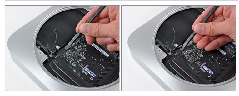
• Use the flat end of a spudger to pry both the hard drive and optical drive connectors up out of their sockets on the logic board.
