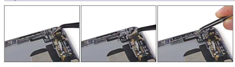
• Pull the hold switch and volume control button brackets away from the rear case to allow access to the button covers.
