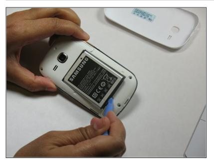
Use the plastic opening tool or your thumb nail to lift the battery out of the receptacle.
