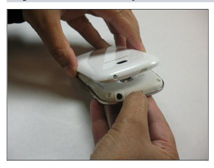
Turn the phone off and completely. Use your thumb nail or a plastic spudger to pry open the back cover,
