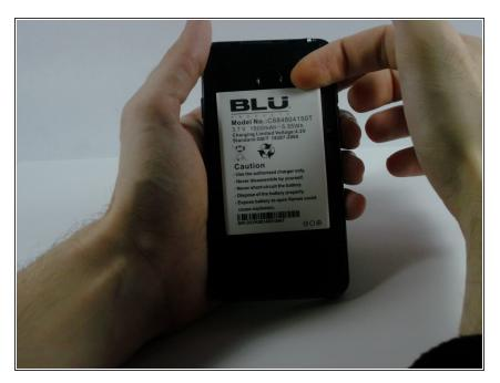
• Use the plastic opening tool or your fingernail to pry off the battery from the top right corner.
