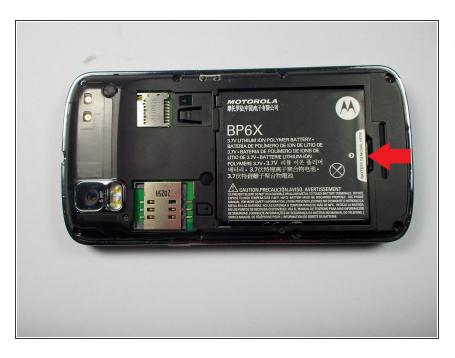
Remove the old battery using the thumb tab then place the new battery in the same position.
