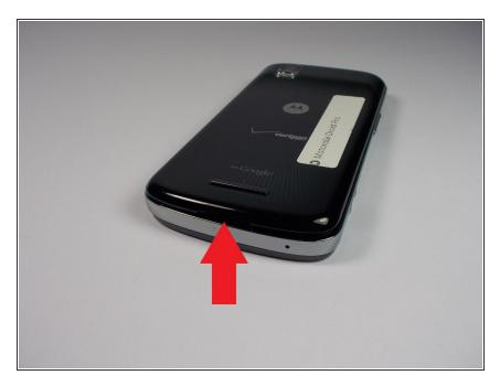
Remove the back cover using the thumb tab located on the bottom of the phone.
