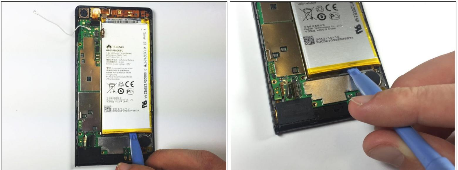
**!** Be careful not to bend, puncture, or crush the battery, even if it is being replaced. The battery can potentially release toxic and flammable chemicals.
