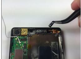
• Use tweezers to lift the rubber alignment tab out of its frame.
