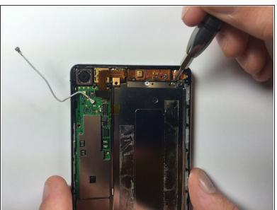
Remove the two 2mm Phillips #000 screws securing the copper flex cable to the silver metal tab.
