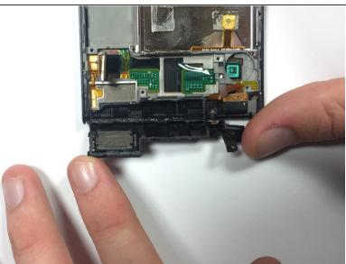
Use the pointy end of a spudger to peel back and fold down the black plastic cover near the bottom left of the phone.
