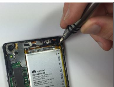
Push down the yellow plastic lining at the top of the battery and remove the two 2.5mm Phillips #000 screws.
