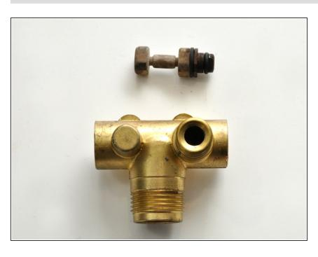
In the interior of the valve, a small plug is pushed to the left and to the right to close the outlet on the right
