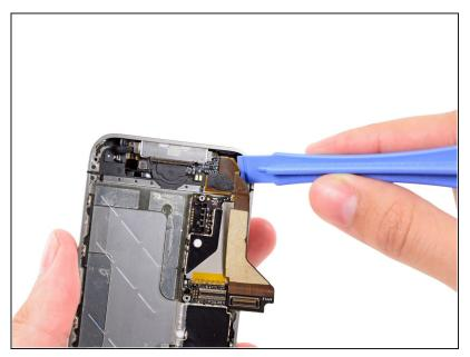
Use the edge of a plastic opening tool to carefully peel the bottom edge of the dock connector assembly off the adhesive securing it to the rear case.
