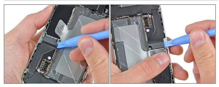
• Use a plastic opening tool to gently pry the dock cable connector up off the logic board from both short ends of the connector.
