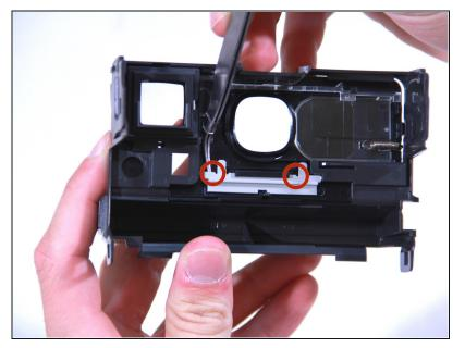
Pry off the slider (the light gray piece) by slipping it out from beneath the tabs (their location is indicated by the two red circles).
