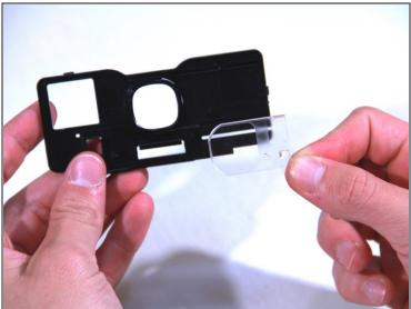
Make sure the last plastic piece is set all the way to the right. Using the blue plastic tool, pry it loose. It should easily pop out.
