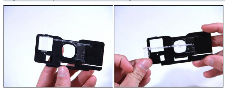
• Slide the CloseUp lens piece all the way to the left. It should separate without any resistance.
