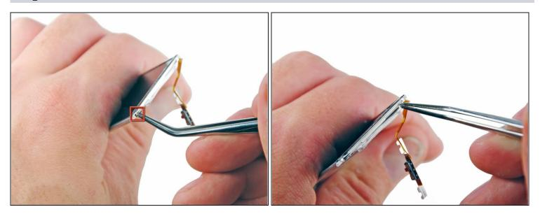
• Use a pair of <u>tweezers</u> to bend back the metal clips at the top of the display.
