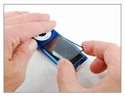
Lifting the glass from the side nearest the top of the iPod, remove the glass panel from the Nano.
