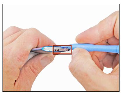
Use an iPod opening tool to pry the hold switch button off of the hold switch plate.
