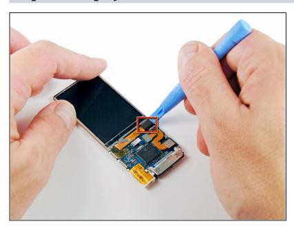
Use an iPod opening tool to pry the display connector off its socket on the logic board.
