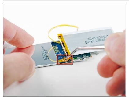
Use a pair of tweezers to remove the orange tape that covers the three solder connections for the battery.
