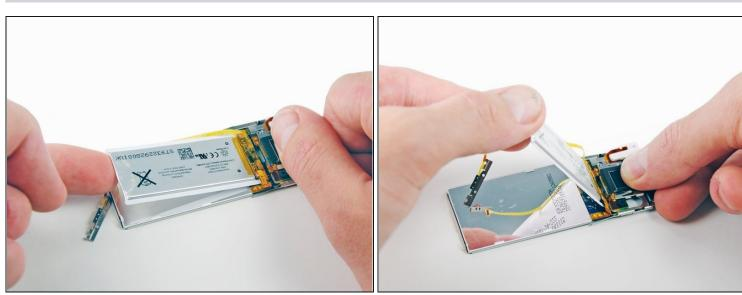
Use your fingers to carefully lift the battery off the back of the LCD, starting at the top
