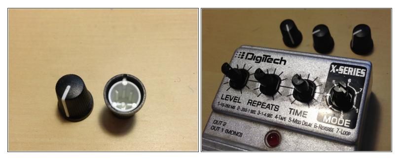
• Remove knobs from the potentiometers by gripping firmly and pulling away from the chassis.
