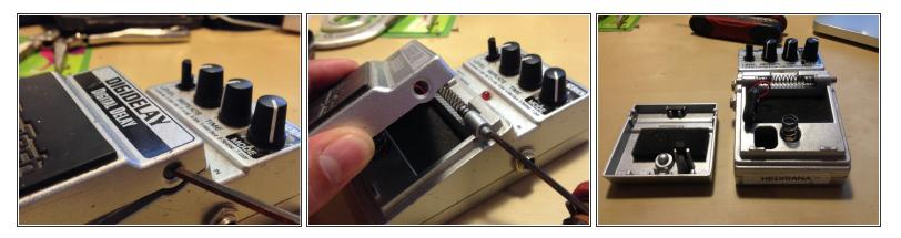
Push in the release pins with an Allen Wrench or the tip of an instrument cable to remove the pedal from the chassis.
