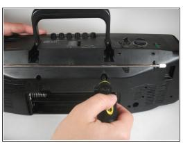
Remove the 6 screws (30 mm in length) with the Phillips #2 Screwdriver from the large holes marked by arrows on the radio.
