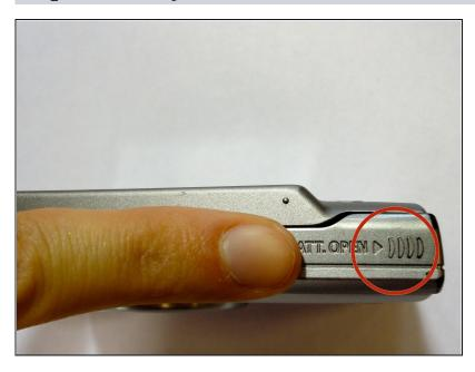
Using your finger, apply light pressure to the grooves at the top right corner of the camera to slide the door to the battery compartment open.
