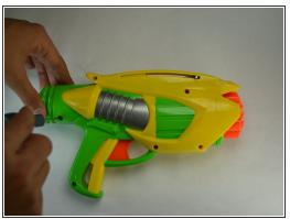
Using a screwdriver, remove the six 9 mm phillips 00 screws holding the main body together.
