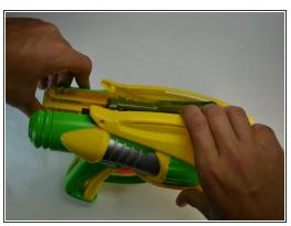
Using the plastic opening tools, carefully take apart the main case of the blaster to leave the inside exposed.
