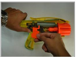
Remove the trigger, lifting from the bottom and pulling it out from under the metal pin.
