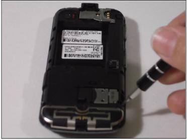
• Remove eight black .4 centimeter screws on the top, bottom, and sides of the phone with a T5 Torx screwdriver by inserting it into the screws and turning it to the left. Set screws aside.
