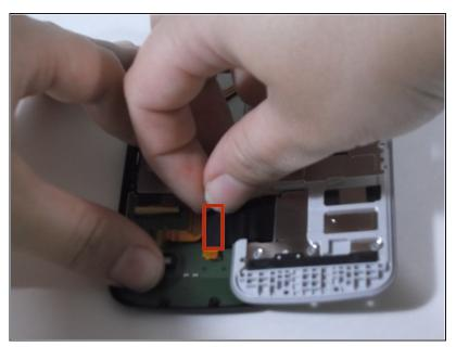
• There will be a short, wide, black strip connecting the two parts. Separate in the same manner as the black and gold strip. Set aside the piece with the strip attached.
