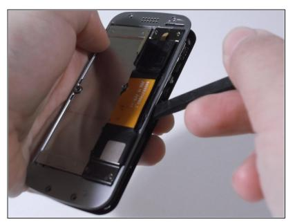
Insert the flat end of a Spudger in between these two pieces of the phone and move it along the sides to loosen and pry apart.
