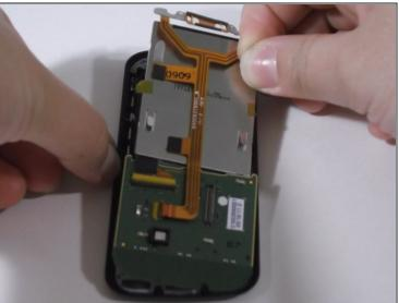
• Peel back the yellow tape on the side of the screen using tweezers or your fingernails. Lift away screen and board.
