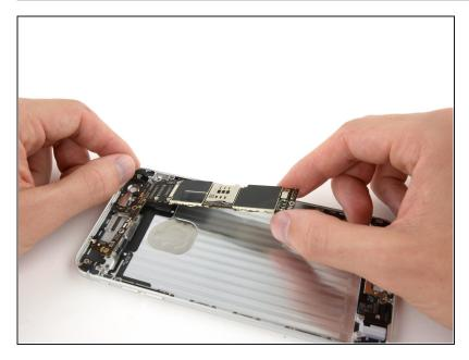
Carefully raise—but do **not** remove—the logic board,
