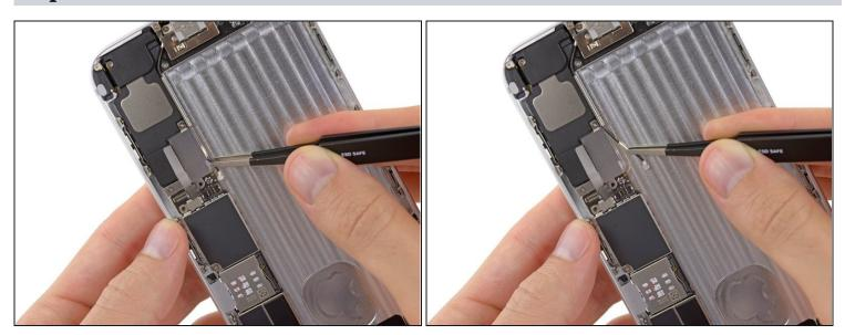
• Grasp the interconnect antenna cable with a pair of <u>tweezers</u> and carefully deroute it from its channel on the speaker assembly.
