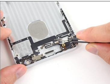
• Use a pair of <u>tweezers</u> to peel the single adhesive tab that resides on top of both the power button and audio control/rocker switch cable connectors.
