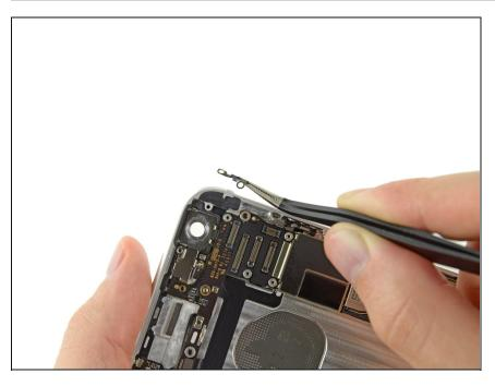
• Carefully grasp the antenna clip with a pair of tweezers and remove it from the iPhone.
