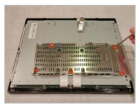
Unscrew the 5 screws holding the metal cage on.
