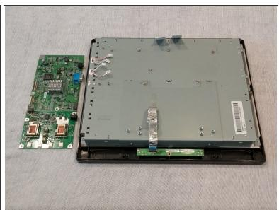
Lift and remove the joined boards.
