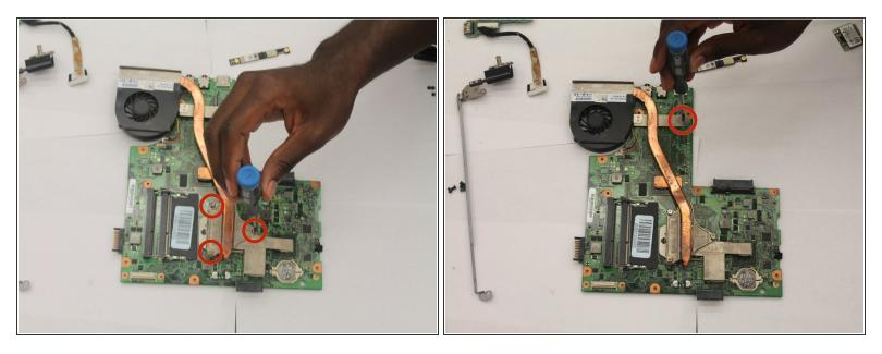
• Remove all 4 of the 6 mm Phillips #000 Heatsink screws with the Phillips #000 screwdriver.
