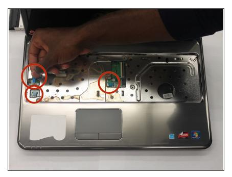
Unplug the palm rest cables by lifting the black tab up and then pulling on the blue tabs.
