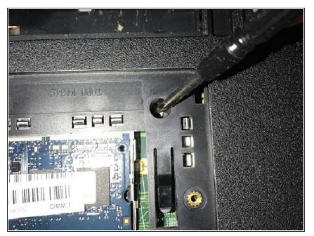
• Remove Keyboard retaining screw from bottom of laptop.
