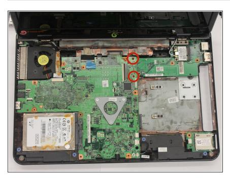
Remove the 4 mm Phillips #000 motherboard screws using the Phillips #000 screwdriver.
