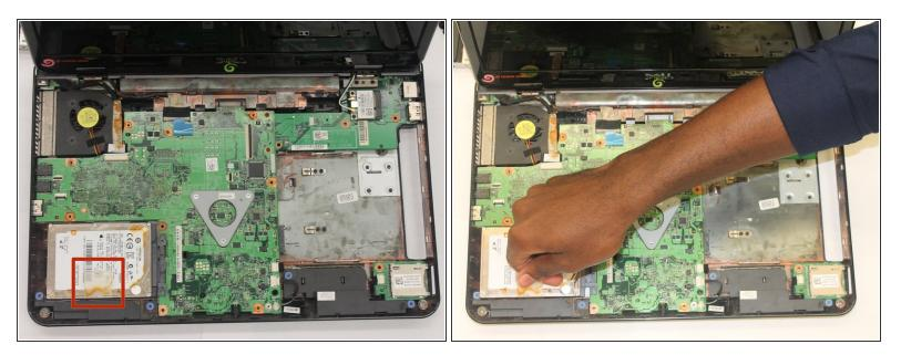
• Pull the clear tab attached to the hard drive and gently lift up the hard drive to remove it.
