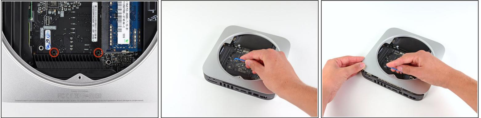
**i** For enough clearance to remove the hard drive, the logic board must be slightly removed. To accomplish this, two cylindrical rods must be inserted into the holes highlighted in red.
