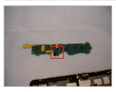
Camera is located in the center of motherboard.
