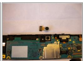
Lift camera and remove from device.
