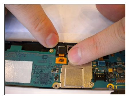
Camera can be found near the top center of device.
