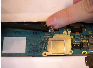
Using Spudger, lift connector from mother board
