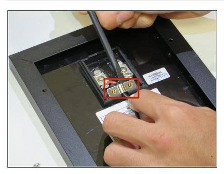
Use the flat-end of the spudger to pry off the clamp which holds the cord down.
