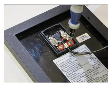
Unscrew the two Phillips #2 5mm screws that hold the power cord in place.
