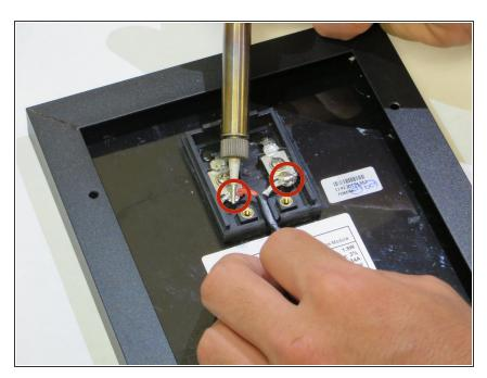
Use the soldering iron to melt down the solder on each terminal by holding the tip of the iron against the solder until it becomes liquefied.
