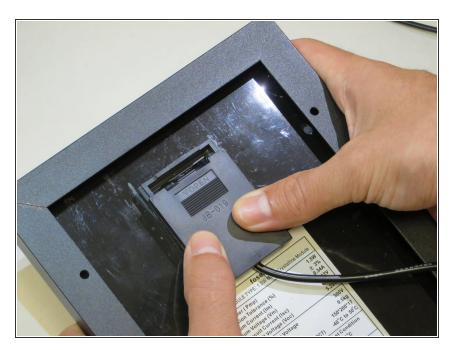
Open the case by pulling the back tab toward you in a downward motion.
