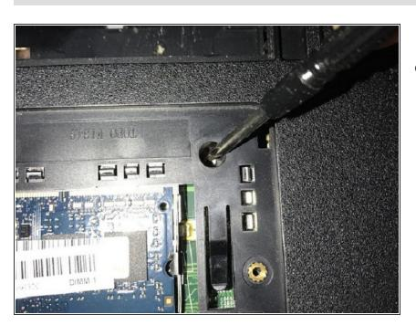
Remove Keyboard retaining screw from bottom of laptop.
