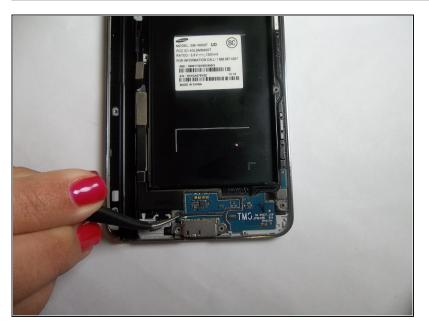
Lift USB port from the front assembly using the tweezers.
