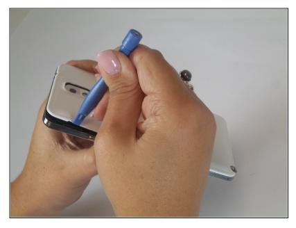
Insert a fingernail or plastic opening tool in the gap between the rear case and the base of the phone.
