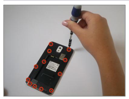
• Remove the twelve 4mm Phillips #00 screws from the back chassis.
