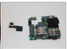
• Using the opening tool, pry up the camera attachment from the motherboard.
