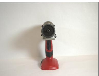
• The threaded hole the screw was in is in the shape of a 6-point star. Insert a T40 Torx Key and rotate it clockwise to loosen and remove the chuck sleeve.
