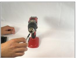
• The chuck sleeve is held on by a 20mm Phillips #2 screw in the center. This screw is reverse threaded. Insert a Phillips #2 screwdriver and rotate it clockwise to loosen and remove it.
