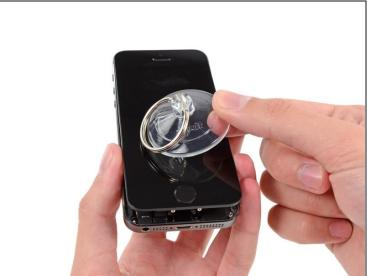
⚠ Do not try to completely remove the front panel assembly from the rear case, as there are several delicate ribbon cables connecting them.
