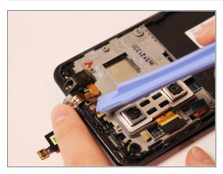
Using the plastic opening tool disconnect the ribbon cable connected to the headphone jack assembly.
