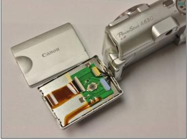
• Gently remove the back panel of the LCD screen
