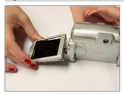
Gently remove front panel of the LCD screen
