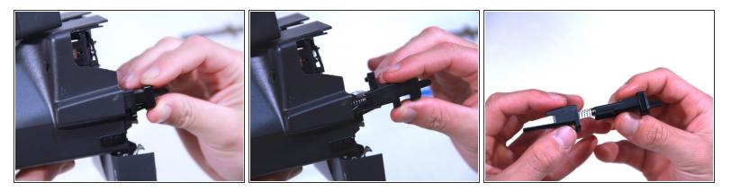
• After the face plate is off, the shutter switch should slide out easily.
