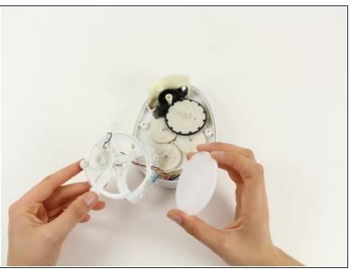
Grab the outside of the large, white gear in the LED housing and pull the gear out of the housing.
