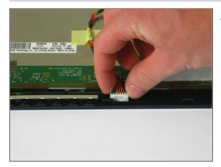
• Grasp the other side of the bundled cable connector and gently pull the connector away from the screen.
